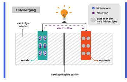
An illustration of a lithium-ion battery during discharge. *Source:* https://www.science.org.au/curious/technology-future/lithium-ion-batteries
