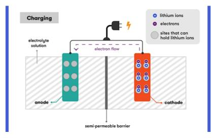
An illustration of a lithium-ion battery while charging. *Source: https://www.science.org.au/curious/technology-future/lithium-ion-batteries*
