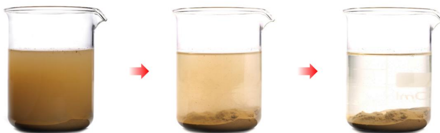
Figure 4.21: Effect of coagulation and flocculation on untreated water.
