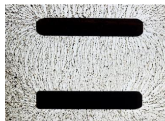
Figure 2.06: Electric field between two oppositely charged parallel plates.
