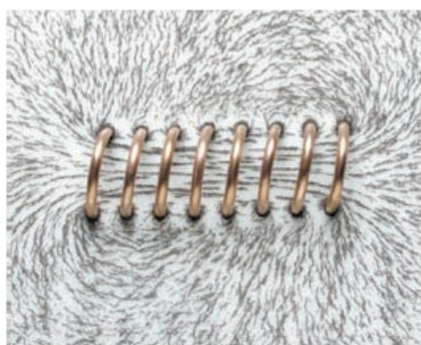
Figure 2.21: Magnetic fields surrounding a straight conductor, a loop, and a solenoid.
